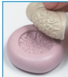
Remove the PMC from the mold and prepare it to be fired.
