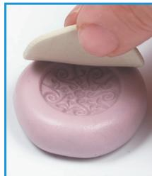
Firmly press unfired PMC® into the cured Rio Cold Mold.
