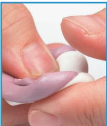
Knead the two parts of the Cold Mold™ compound until the color is uniform.
