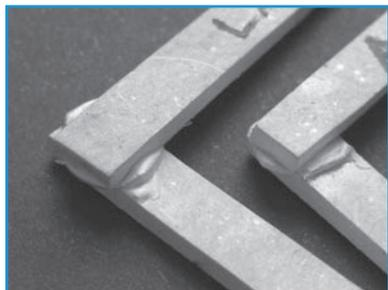
This close-up shows two of the brackets after firing. In each case, an equal and generous puddle of paste was used to make the joint.
