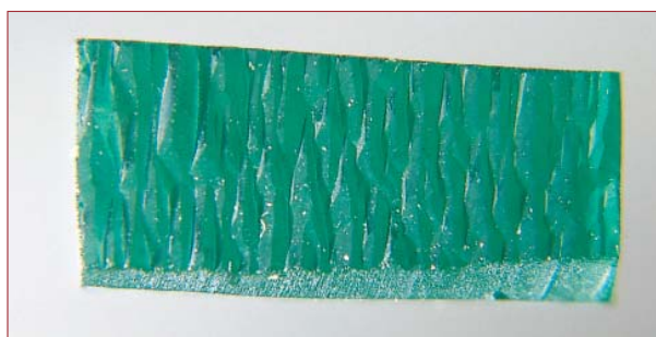
Figure 7: Rough crystal plate of 7.52 ct the new type of Tairus hydrothermally-grown synthetic emerald coloured by vanadium and copper showing an uneven, undulating surface formed by numerous faces of subindividuals of synthetic emerald; size of plate about 16.5 × 7.5 mm, weight 7.52 ct. Photo by M. Glas.
