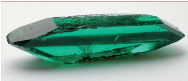
Figure 5: A typical synthetic emerald crystal measures about 80 \times 18 \times 14 mm. Courtesy of D. Fursenko.
