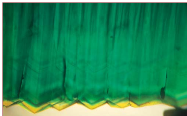
Figure 14: Rough crystal plate with step-like growth lines and colour zoning, irregular subgrain boundaries almost perpendicular to the growth and colour zoning. Immersion, 40×. Photo by K. Schmetzer.
