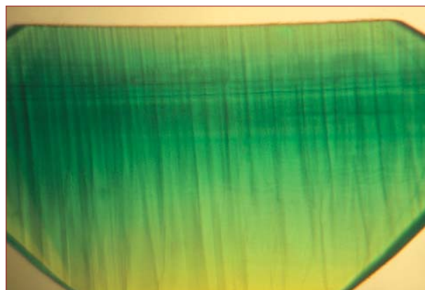
Figure 13: Faceted Tairus hydrothermally-grown synthetic emerald coloured by vanadium and copper; with step-like growth lines and colour zoning, and irregular subgrain boundaries almost perpendicular to the growth and colour zoning. Immersion, 40×. Photo by K. Schmetzer.
